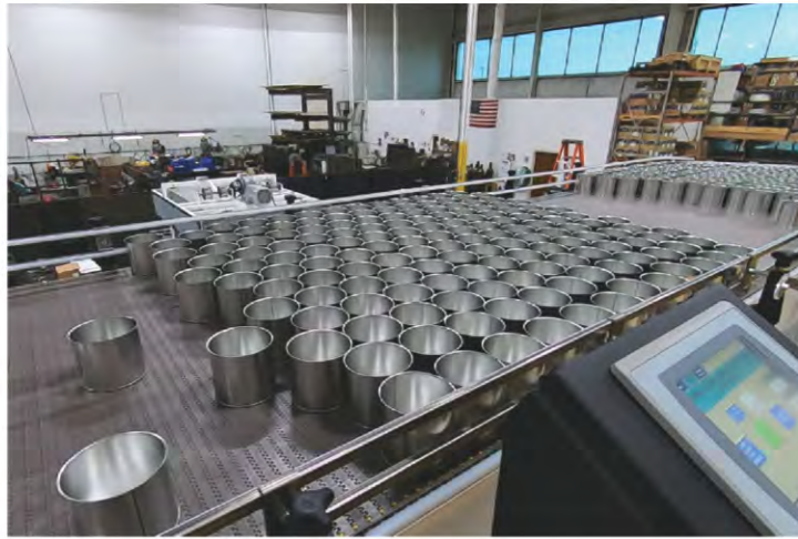
The PLC allows for multiple container recipes/ presets to be added for ease of changeover between container types of the same material on the FHA 3000 depalletizer
