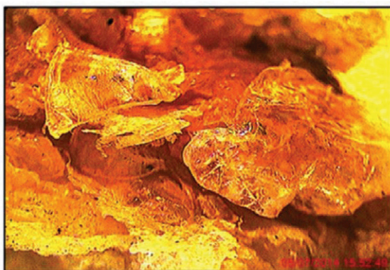
Incompatible PP/PET/PE— No Additive
