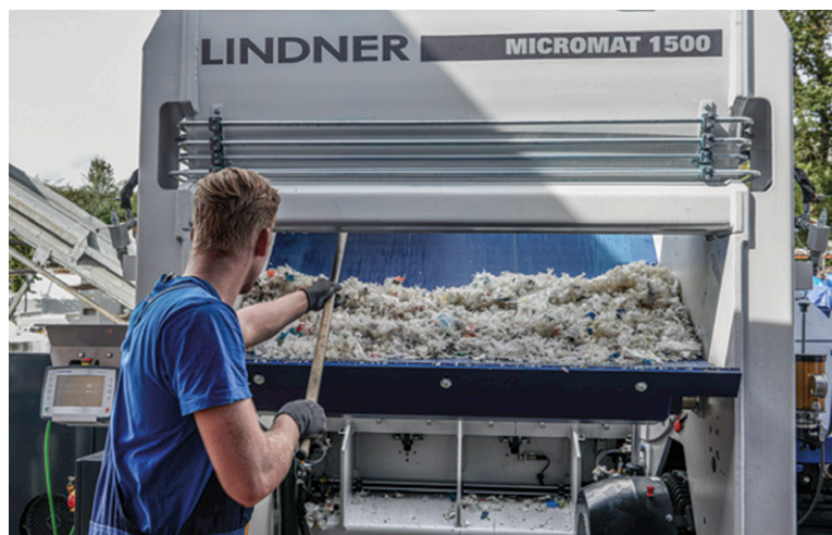
Above: The Micromat 1500 from Lindner Recyclingtech
