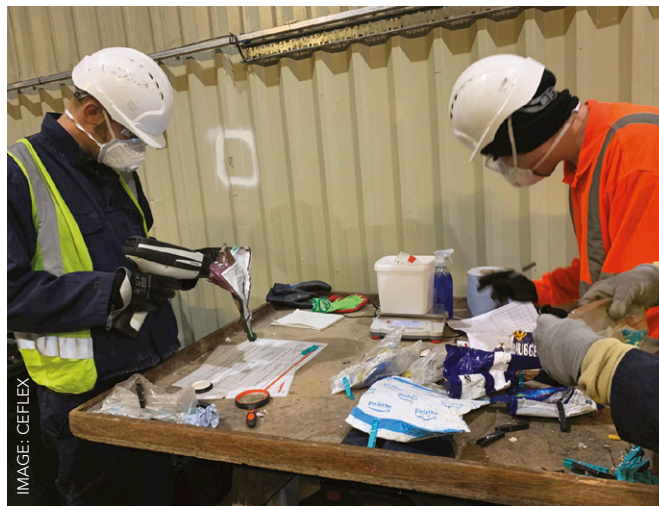
Researchers are using NIR scanners to identify plastic materials
