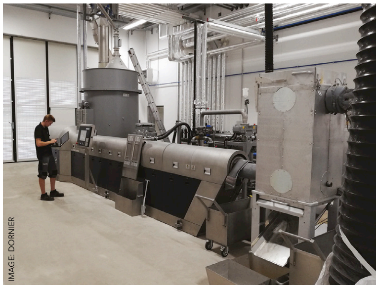
Above: The recycling of production waste in the manufacture of BOPET biaxially oriented films is already common practice, but Erema says production becomes an extra challenge if PCR is also used. It worked with Lindauer Dornier to fulfil a customer's requirement by integrating components for the first time in a recycling line for a film manufacturer in Europe. The line combines an Erema Intarema 1512 TE recycling machine with a Lindauer Dornier melt filter for fine filtration
