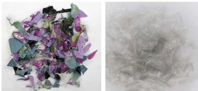
Above: Flexible packaging waste-printed LDPE before (left) and after (right) Sorema's de-inking process
