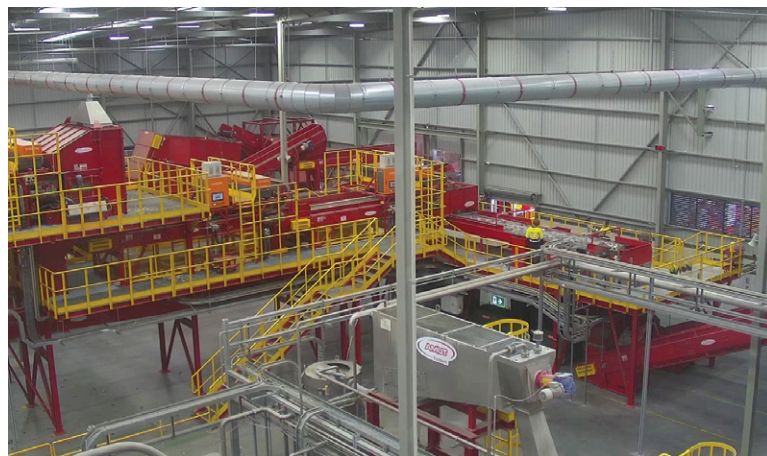
Above: Amut supplied the post-consumer PET bottle sorting and washing line at the Albury facility in Australia
