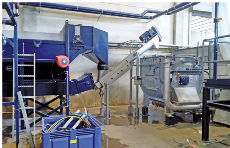
Above: PP flakes in Herbold Meckesheim's washing plant are transported as floating material with a dewatering screw to the downstream mechanical dryer
