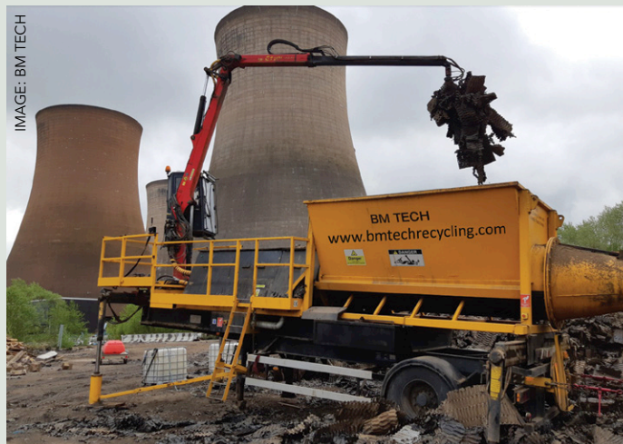
Left: BM Technology Tech in the UK recovers, cleans and chops rigid PVC
