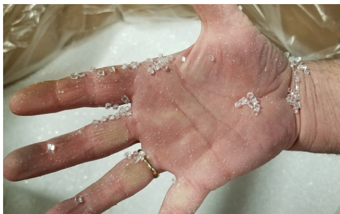
Above: Dust is commonly produced during pellet cutting and conveying (left). BPM's pellet evacuation system and dedusting cyclone results in a marked reduction (right)
