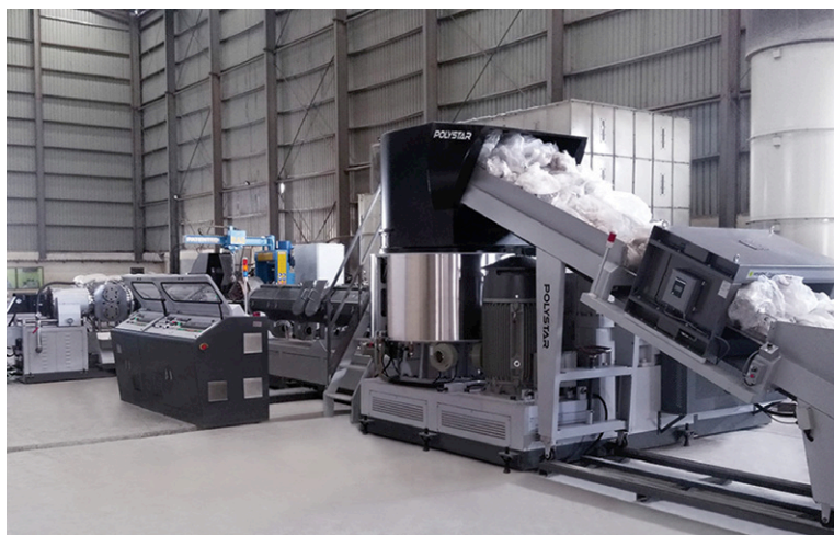
Above: Post-consumer film recycling line from Polystar
