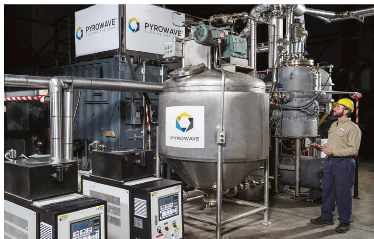
Above: Pyrowave has developed "catalytic microwave depolymerisation" technology for polystyrene
