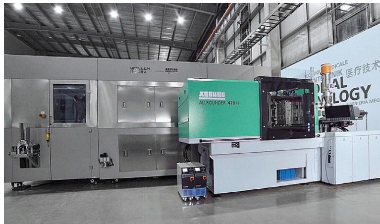
Above: A hybrid Arburg Allrounder 470 H with a hot runner mould produces 48 tips per 6-second cycle
