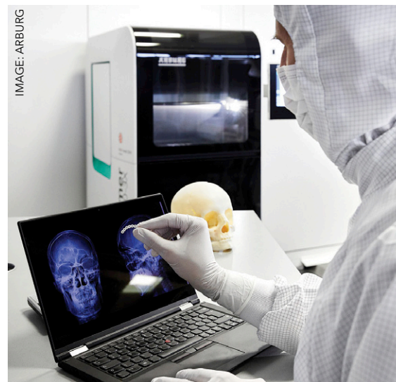
Above: Arburg's Freeformer for additive manufacturing has a large potential for medical technology. The machine can be used in cleanrooms and processes FDA-approved original plastic materials
