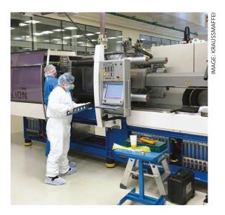
days so as to ensure compliance with the required ISO 7 cleanroom class through a reduced particle discharge. It was then delivered to Weidmann at the end of April. Following its commissioning in the cleanroom, it was ready for production within just a few days.
