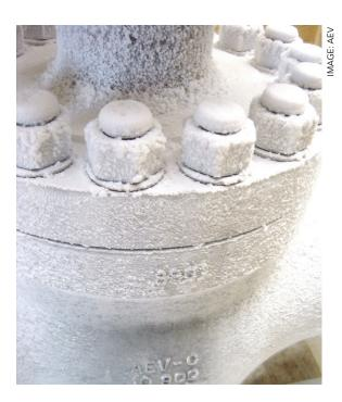
performance cryogenic PEEK polymer to help its customers operate applications more efficiently and safely. The company's 2XC\* C-ball valve products require zero maintenance in cryogenic service.
