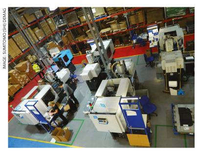
Above: UK-based Hi-Technology's dedicated precision moulding cell, with Sumitomo (SHI) Demag machines, provides additional flexibility to support customers in the critical respirator, PPE and medical pump sectors
