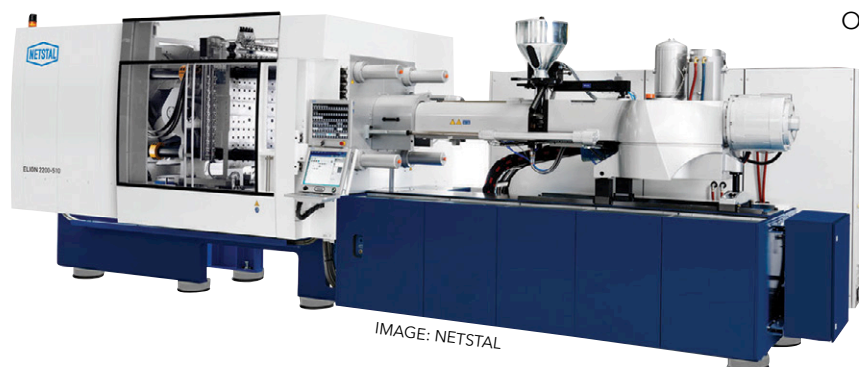
Above: An all-electric Netstal Elion 1200 is producing pipette tips at K2022
