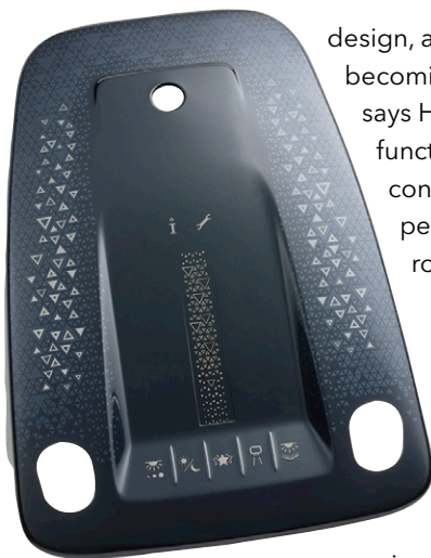
Above: Overhead lighting console incorporates numerous decorative and functional features
