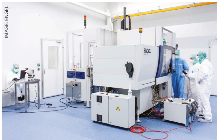
Above: Cleanroom production at Helvoet in the Netherlands. The company specialises in precision injection moulded products and uses all-electric E-mac injection moulding machines by Engel
