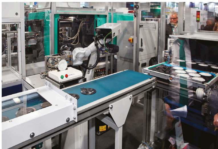
Above: Functional testing station during production of a nightlight incorporating TactoTek technology on the Arburg stand at K2019
