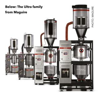
proved auto start and auto stop features. "When you want the dryer to stop drying a grade of material at 6pm, it will automatically stop at that time, but most importantly it will stop empty, so as to allow a very rapid and efficient clean-down process, and then a fast start-up of the next grade," says Crittenden.
