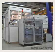
Injection moulder Hans Geiger has developed an enclosed production line for products used in the manufacture of circuit boards
