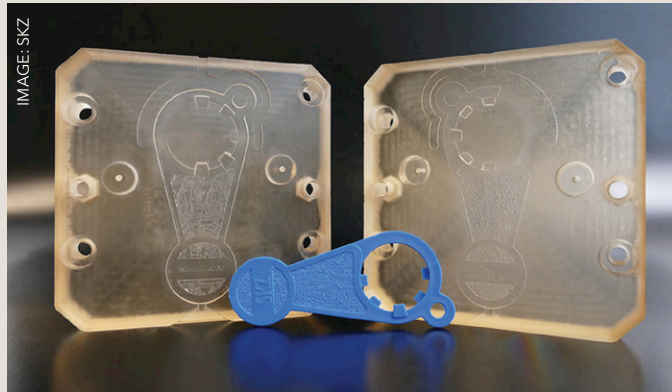
Left: 3D printed tool inserts produced in the SKZ ADDfoam project
