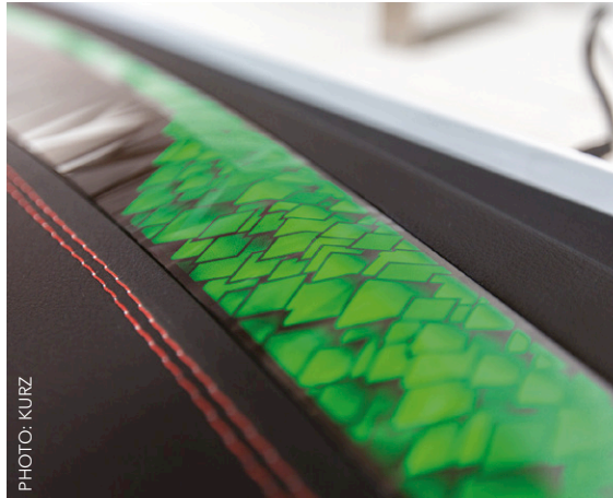
Left: Door trim with day/night design and touch-activated backlighting
