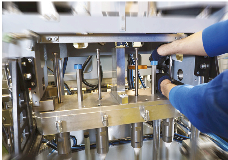
Above: Sipa has introduced a new quick mould change system for its ECS SP single-stage injection-stretch-blow moulding machines. The system is capable of producing all sorts of shapes, including the production of miniature bottles as small as 10 ml in size
