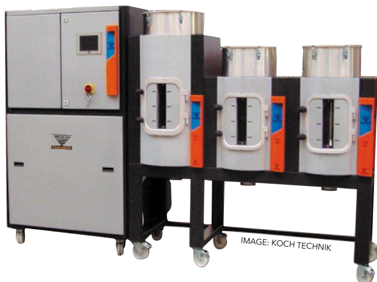
Above: EKON is a new type of dry air dryer from Koch-Technik that combines the CKT and EKO drying concepts
