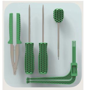
Above: Solvay's Ixef GS-1022 PARA forms the awl and pin-screwdriver handles, measuring calliper, and locking plier handles in Intelligent Implant Systems' kit. The polymer's high impact resistance also eliminated the need for a metal strike plate that had been part of the awl's early designs. This reduced cost and simplified manufacturing.
