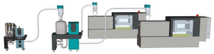
Above: Image shows the Somos Perfoamer units from ProTec for drying and temperature adjusting polymer pellets, loading them with CO2 under pressure and then feeding them to the injection moulding machine. Photo: ProTec Polymer Processing
