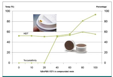
With increasing BioPBS content in a blend with PLA, the level of crystallinity increases rapidly after the addition rate rises above 20%, hitting 50%, before it virtually plateaus, hitting a maximum at an addition rate of 80%. Additionally, when using 60% of BioPBS and more, heat deflection temperature, HDT, sharply increases to almost 100°C
