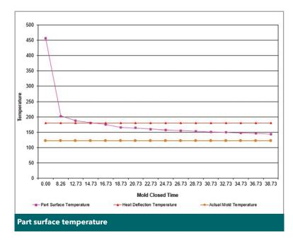
temperature of the part was measured several times over a 2-hour run at 74°C.
