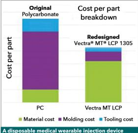
made in PC was redesigned for manufacture with Celanese's Vectra MT LCP, reducing system cost
