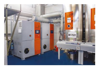
Above: Motan-Colortronic's installation at Mitschke included two interconnected dry air generators equipped with **ETA Plus air** volume controls, a dew point control unit and a water cooler for the return air
