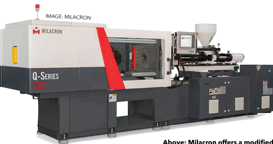
Above: Milacron offers a modified Q-series 610 model for the production of pails. It has a faster clamp, higher torque extruder, quicker ejector, extended L: D screw and updated water and air connections
