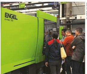
Right: In Shanghai, Engel demonstrated how a twocompartment yoghurt cup including IML decoration can be produced economically and efficiently on an all-electric E-mac 180 injection moulding machine
