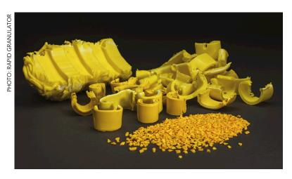
Above: The steps from lump to chip to quality regrind with Rapid's Raptor Duo concept and efficiently re-purposed in the manufacture of new products."
