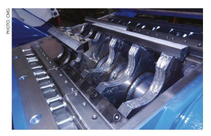
Above: Granulator cutting chamber with **U&G** blades from CMG
