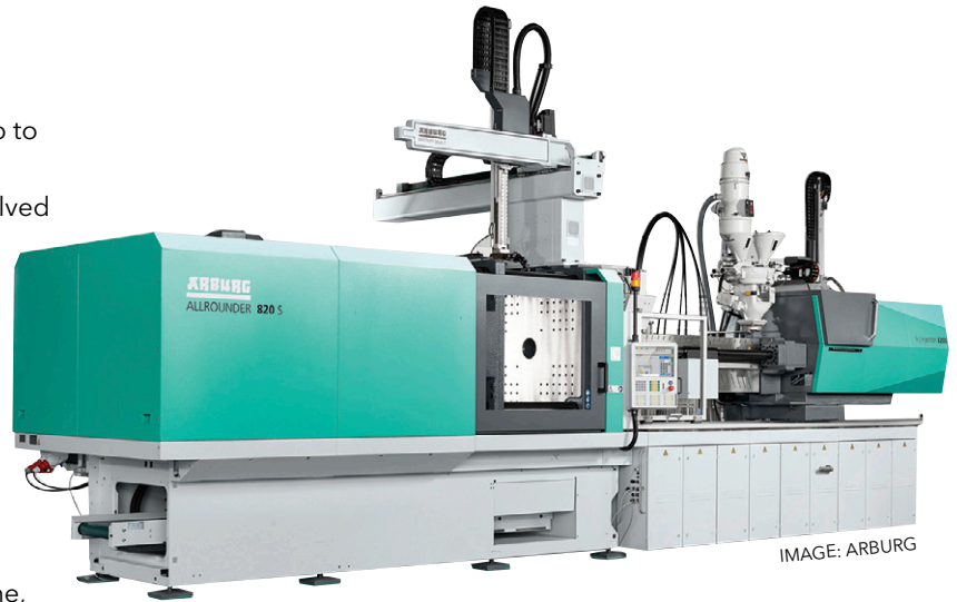
Above: The Fibre Direct Compounding process from Arburg enables inline compounding on an injection moulding machine, which allows the use of long-fibre materials, as well as combinations with continuous reinforced fibres
