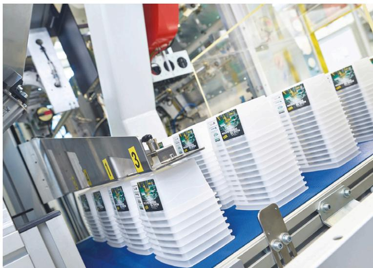
**Above left: Arburg's hybrid Allrounder 820 H in the "Packaging" version debuted at Fakuma 2018. Above right: At the event, Arburg's hybrid Allrounder 820 H produced thin-walled IML containers in a four-cavity mould in a cycle time of around 3.8 s**
