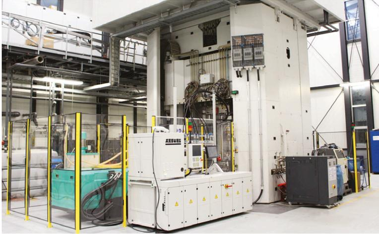
**Above: A specially-designed Arburg injection unit with integrated Fibre Direct Compounding can be quickly connected to and disconnected from a Dieffenbacher vertical press**
