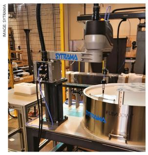
Above: Photo shows an innovative system from Sytrama that provides an alternative to the standard solutions of cup vibrators used for loading inserts into the mould (in this case, filters for respiratory masks). It consists of a rotating bowl that distributes the inserts and SCARA robot with a vision system that sends the coordinates of the piece to be picked up by the robot
