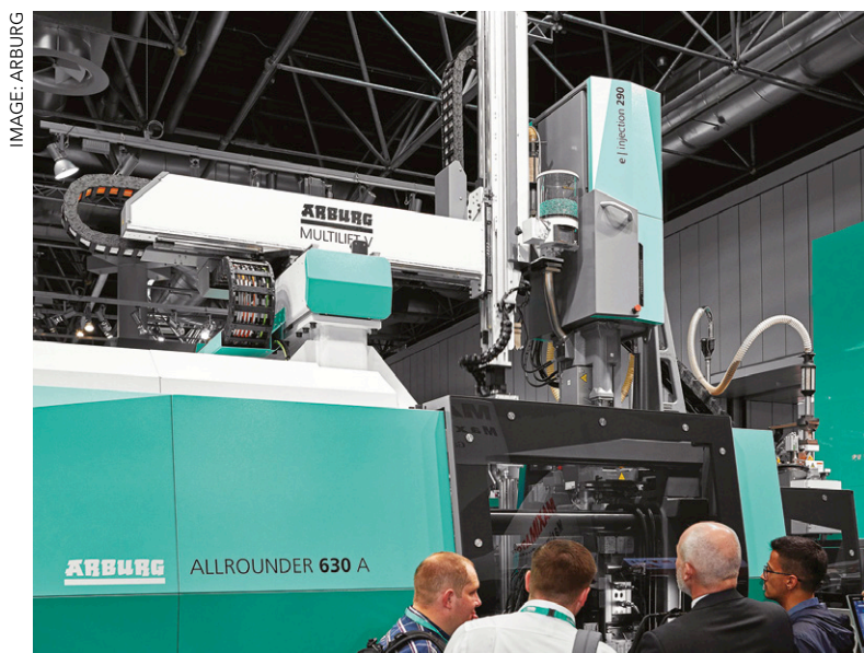
Above: The new Multilift V30 expands Arburg's portfolio of linear robotic systems, designed for large injection moulding machines. The turnkey solution described produces two-component handles for Allrounders. The handling is performed by a six-axis robot
