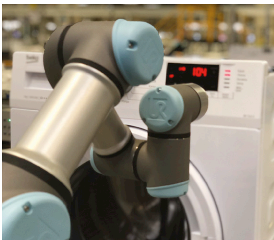
Above: At Arcelik Group, even the function check of the manufactured washing machine is largely automated. Only the control knobs are tested by people because machines may have difficulty assessing their haptics
