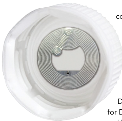
Above: A new packaging solution, Talkin' Cap, uses embedded Near Field Communication tags, for application on the inside of closures from CSI
