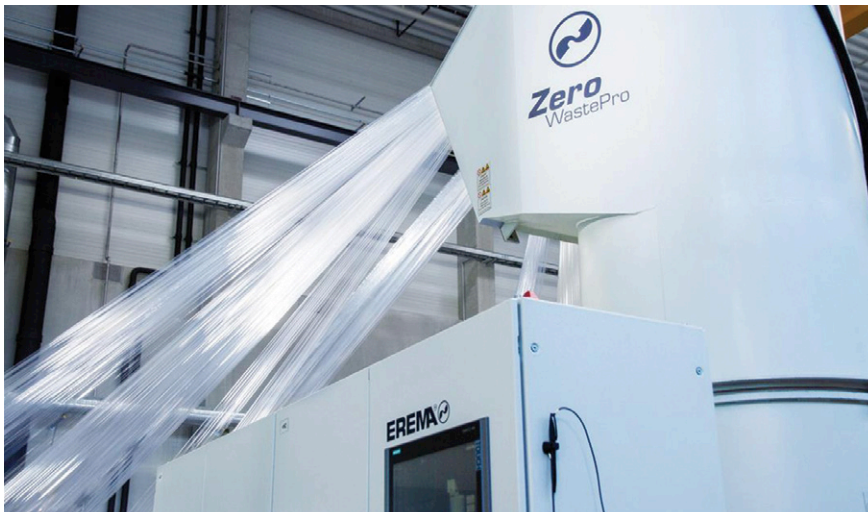
Above: Erema's Intarema ZeroWastePro is used to recycle PE and PP film
