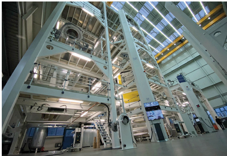
Above: Kuhne's Triple Bubble blown film lines can be used to make ultra-thin thermoforming film
