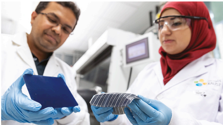
Above: Kaust researchers have combined silicon solar cells with a polymer backing to create devices that combine flexibility with high efficiency
