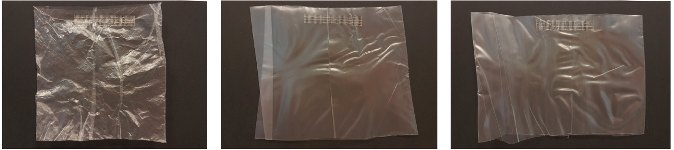
Evonik trials show (left-right): a PP film structure without PPA; with fluorine-based PPA; and with 1% non-fluorinated Tegomer 6850
