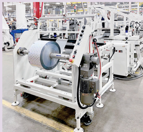
Right: Hudson-Sharp has added dual-registration to its Ares 400-SUP machine
