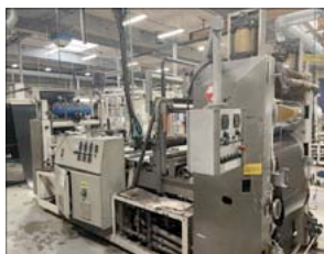
1040mm wide Welex 3 roll polishing stack
