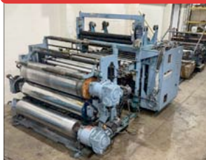
2290mm wide Davis Standard sheet extrusion line
