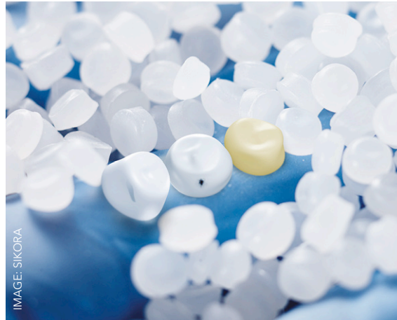
Left: Sikora's Purity Scanner technology detects a wide variety of contaminants in polymer pellets
