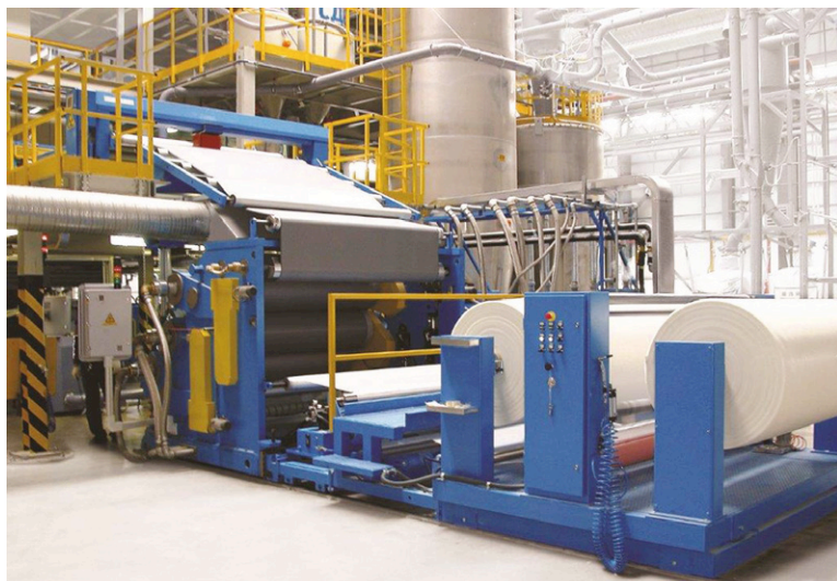
Above: Amut will highlight its extrusion lines for PVC and TPO waterproof membranes
