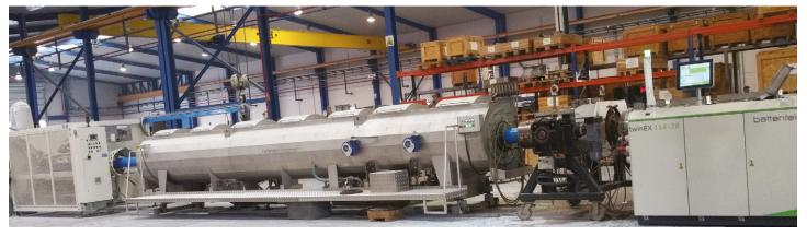
O-PVC pipe extrusion line with twinEX 114-28D extruder (© Molecor)
