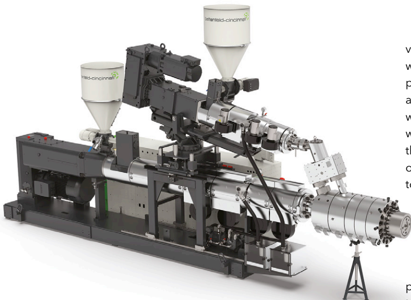
Above: Battenfeld-Cincinnati's new three-layer Spider NG 250-3 pipe head is suitable for pipes from 110 to 250mm in diameter
