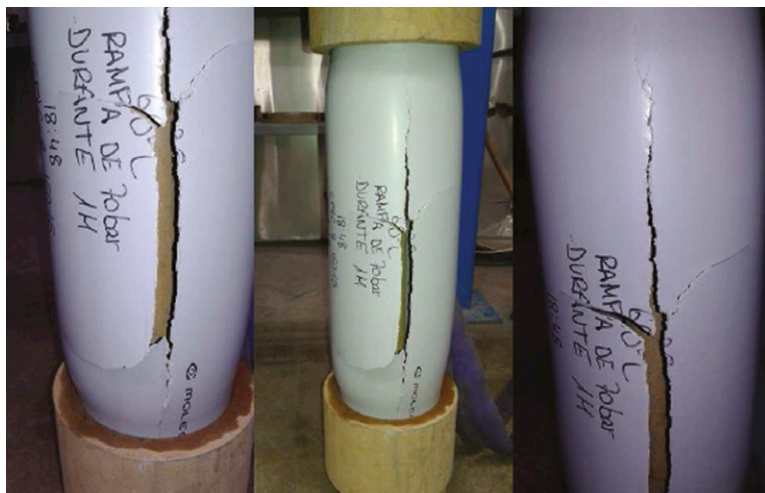
Above: Molecor has tested the effectiveness of creating oriented chlorinated PVC for pipes
