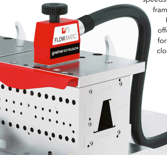
Left: During K2019, Greiner Extrusion produced a hollow chamber profile on a line including its FlowMatic system, which controls filling within the die
