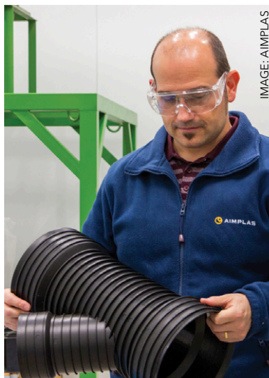
Above: Life Circ-ELV has produced pipes and fittings from recycled car bumpers and fuel tanks
