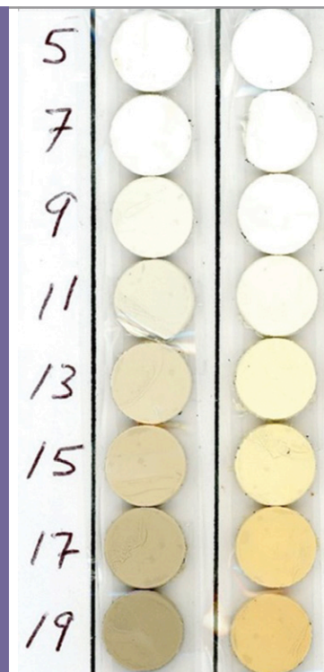
Figure 1: Brabender chips for a Therm-Chek Ca/Zn organic based stabiliser developed as a tin offset for substrate formulations. The Ca/Zn powder system (right) shows the early colour that tin stabilisers are known for along with improved mid-term colour and no loss of processability. Left column shows time in minutes
