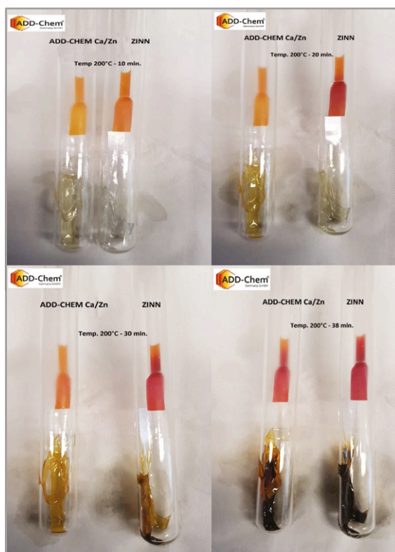
Figure 3: Effect of heat on clear PVC stabilised with Add-Chem's Ca-Zn stabiliser compared with a tin alternative after 10, 20, 30 and 38 minutes at 200°C (the colour change of the Congo Red paper indicates halogen release)
