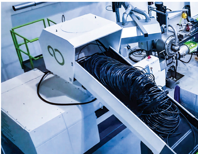
Above: Pure Loop says its shredder-extruder combination, plus laser filter, makes recycled pellets during irrigation pipe production
