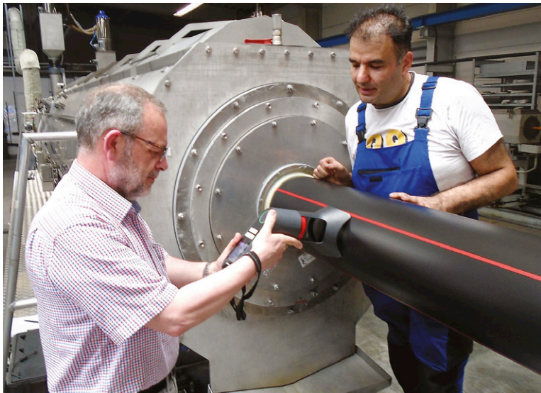
Above: WKT is using handheld Warp technology from Inoex to check the thickness of its PE pipe
