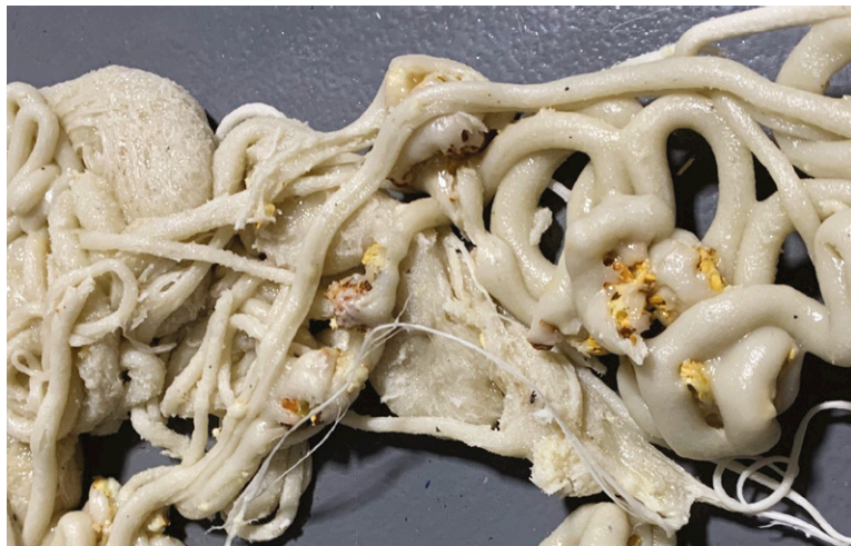
Above: A purging compound from Asaclean after a full machine purge showing the captured contamination
