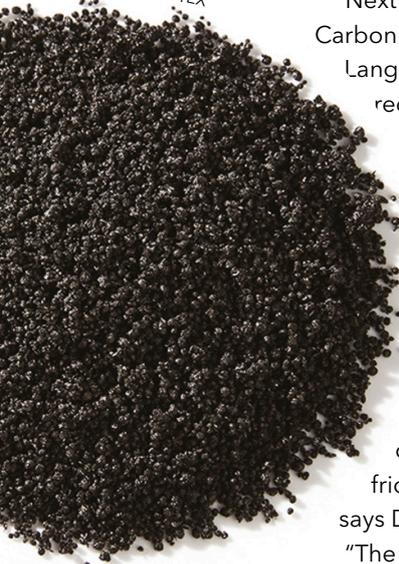
**Above: Procotex subsidiary Apply Carbon has expanded capacity for production of its granular recycled carbon fibres**
