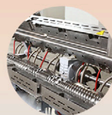
Clamshell Barrel Co-Rotating Twin Screw Extruder [ Diameter : 16mm - 135mm ]
