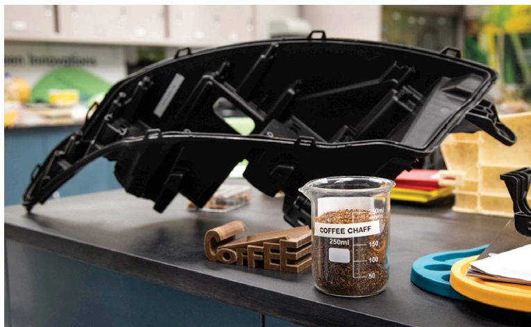
Above: Ford replaced a 40% talc filled PP with a 20% coffee chaff filled PP alternative in this headlamp housing for its Lincoln Continental, estimating a 5% cost saving, 17% weight saving and 25% reduction in process energy
