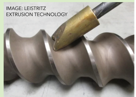
IMAGE: LEISTRITZ EXTRUSION TECHNOLOGY Above: An impact gun with a brass tip can help loosen stuck screw elements without risk of damaging elements or shafts
