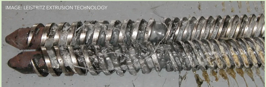
IMAGE: LEISTRITZ EXTRUSION TECHNOLOGY Above: Removing elements for cleaning or screw reconfiguration can be simplified using a structured approach
