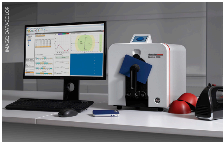
Above: Datacolor's latest Spectro 1000 model measures sample colour and temperature
