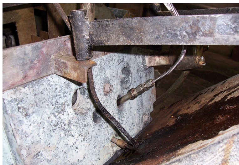
Below: Equitech's IPS system uses ruggedised fibre-optic probes for direct measurement in the melt stream of an extruder
