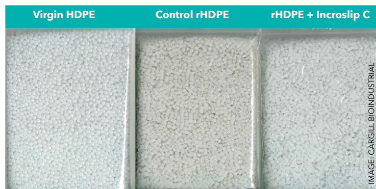
Above: HDPE pellet samples show the whiter colour that can be achieved when using Incroslip C
