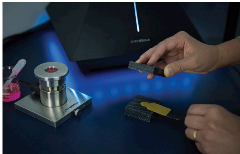
Above: Testing thermal conductivity of a carbon fibre composite using C-Therm's Trident equipment
