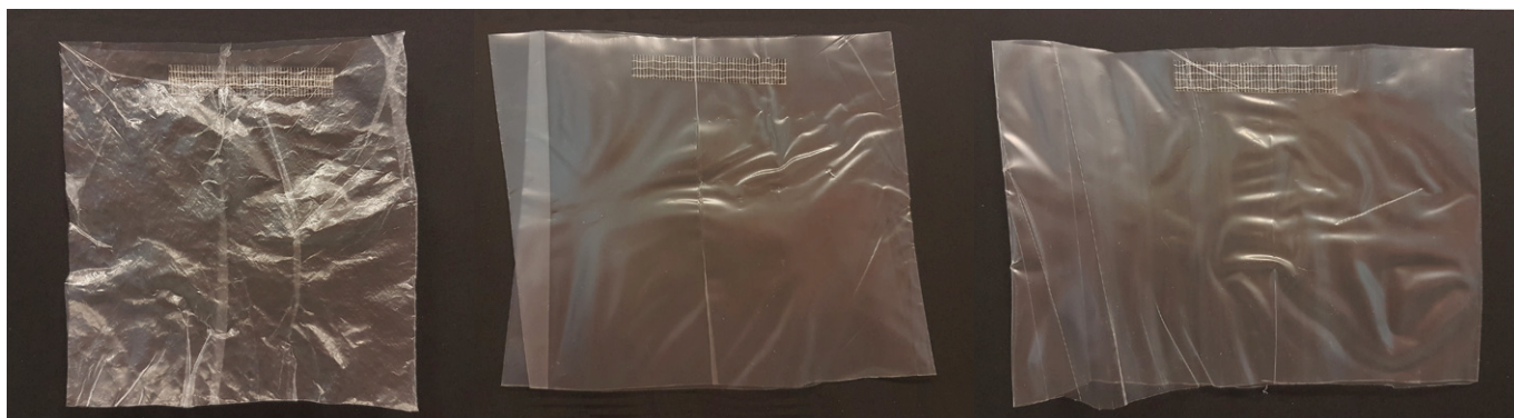
Above: Images show the surface quality of PP films without a processing aid (left), with 1% of a fluorine-based masterbatch (centre), and with 1% of Evonik's Tegomer 6850
