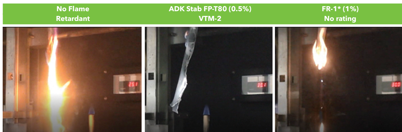
Above: Images showing UL94 VTM (Vertical Thin Material) fire resistance testing of a 200-micron MFR 2 LLDPE film with no flame retardant, ADK Stab FP-T80, and a competitive traditional NO-Alkyl FR
