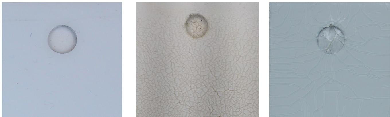
Above: Images showing an unaged sample of a transparent construction film (left) compared with the same film after 180hrs exposure in an Eye Optix Super UV system (centre) and to 24 months of Florida sunshine (right)
