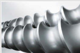
STS Mc 11 - the next generation of Coperion's STS twin screw extruders. Featuring a specific torque of 11.3 Nm/cm 3 .
