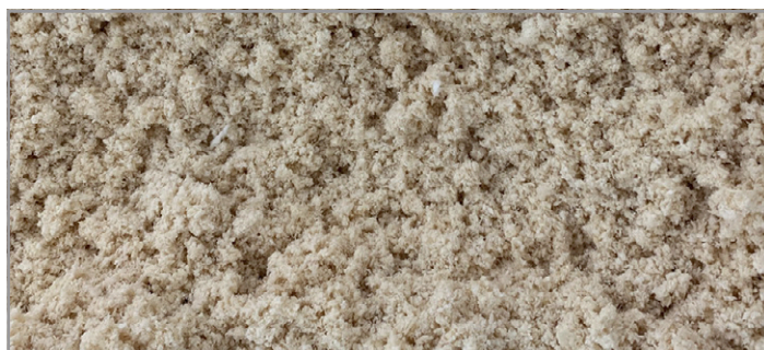
Figure 1: To create a blend of 60% PLA with 40% cellulose fibre, such as that shown above, Mixaco's HM/KM Wood system regulates parameters including hot mixer rpm (blue), hot mixer temperature (red), and hot mixer torque (green)
